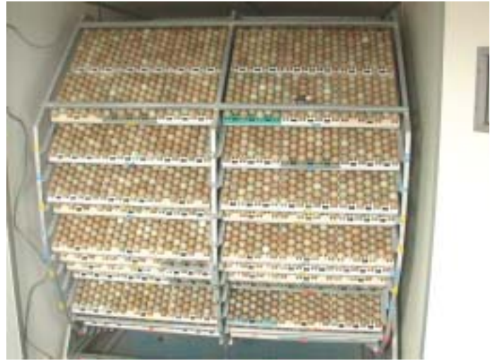
This is one of three incubators that the Krugs have. These incubators each hold 22,000 eggs, which will hatch in 21 days. This room is environmentally controlled to provide exact heat, 99.5 degrees constantly.
